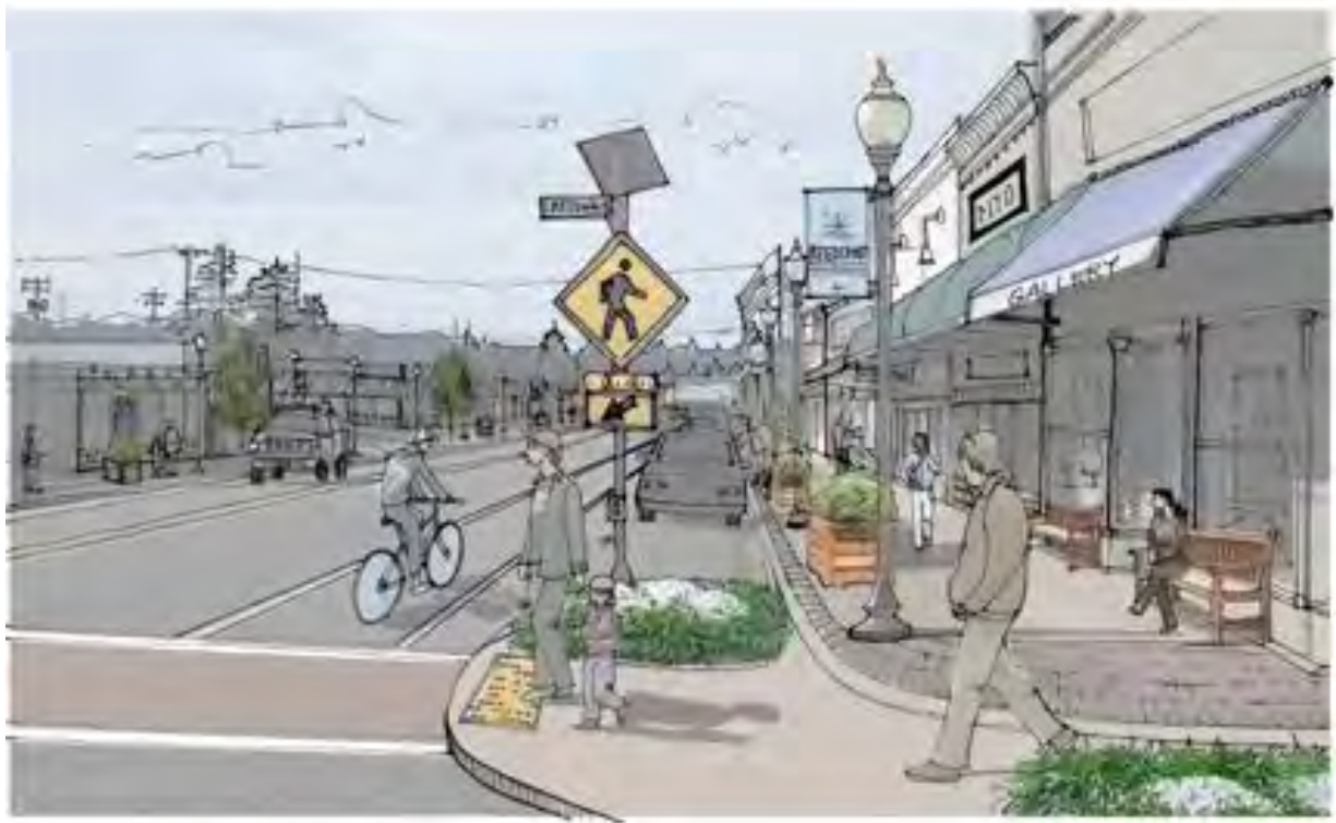
Figure 14 gives a typical downtown street section with curb extensions that “shadow” or match parallel parking width.
