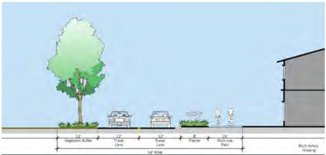
Figure 10 East Railroad Avenue Typical Section
